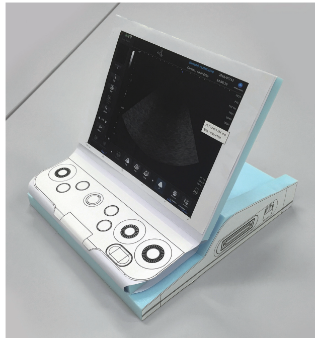
Fig. 2 Mock-up model of SONIMAGE MX1 at early stage of development.
